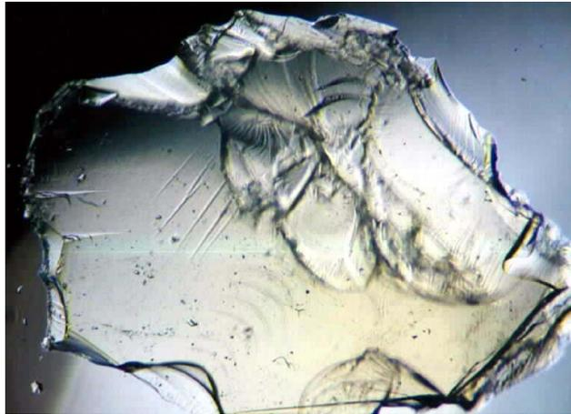
Figure 2 : Transparency of silica aerogel
